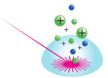
**DNA IONIZATION:** The analyte crystals are irradiated by a laser, inducing desorption and ionization of the molecules
